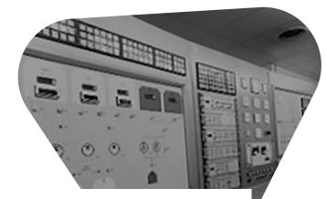
Modular construction based on racks (19 inch)
